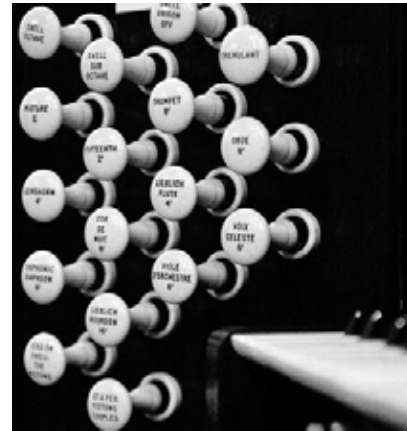
On an organ, different sets of tonal sounds are controlled by STOPS.
